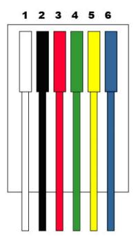
When testing RJ12 phone cables: Tester will test each pin sequentially. Green LED will illuminate for phone cables starting at pin 1 and ending at pin 8. Cable is GOOD when all green LED's light up in sequential test order:
