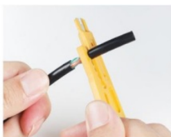
Stripping network cables
