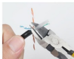
Cut the plastic core
