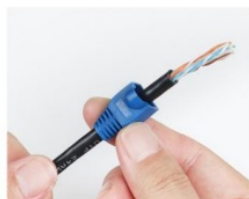
Install strain relief boots
